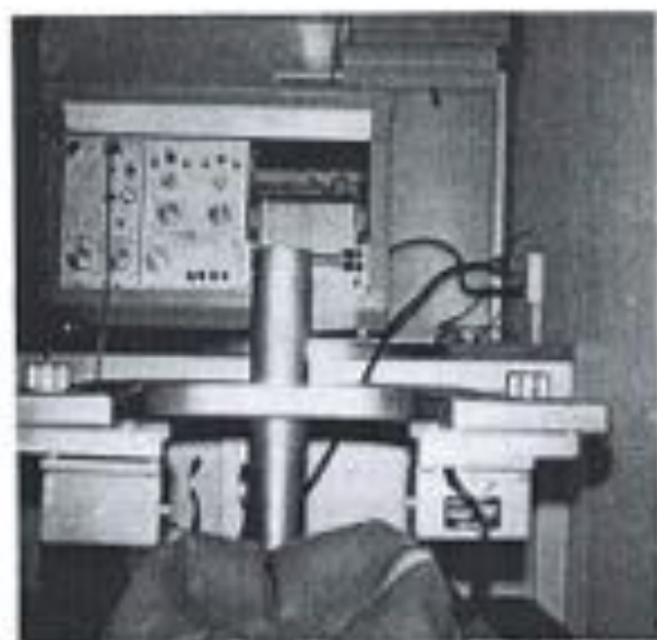
Fig. 2. Close-up of apparatus, showing joints and coupling yokes.
